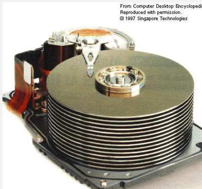
Figure: Magnetic disc (Pic: [img.zdnet.com](http://img.zdnet.com))
