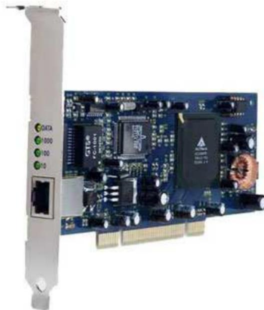
Figure: Ethernet board (Pic: [cache.gizmodo.com](http://cache.gizmodo.com))
